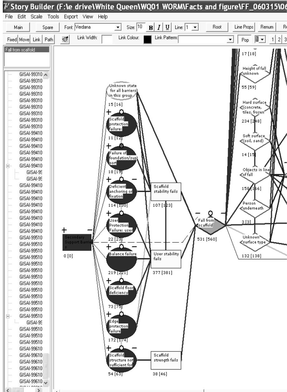
Figure 2 Part of collapsed structure for storybuild: Fall from height scaffold.
